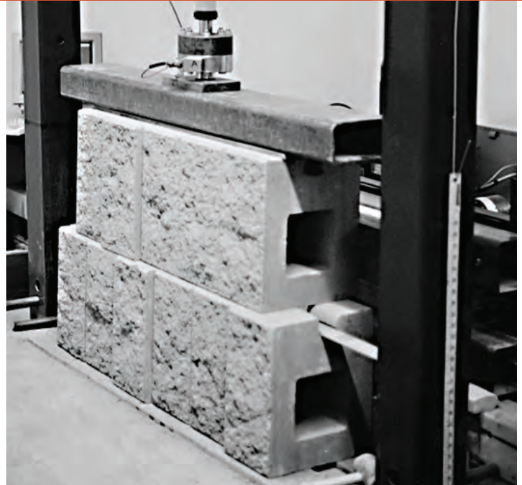
Connection test apparatus with Landmark® modular units.
