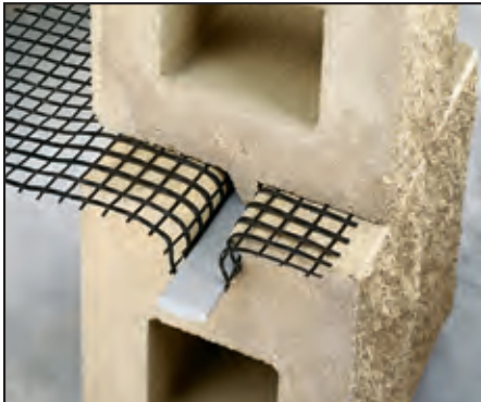
The patented, polymer-based lock bar mechanically clamps the geosynthetic reinforcement to the Landmark block.
